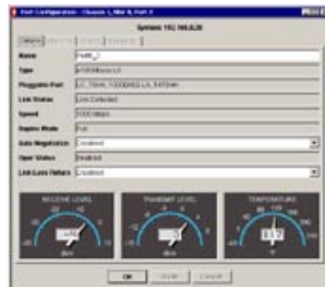
Quality of Optical Amplitude: Real-time measurement of the receive and transmit levels of the optical transceivers. Acts as integral power meter.
